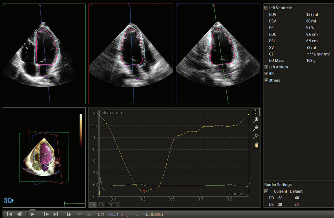
Figure 4 Dynamic HeartModel A.I. application five-up display showing the dynamic contours on the automatically aligned AP4, AP3 and AP2 views along with the volume waveform.
